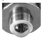
Step 8: Insert the spring into the Quartz sleeve and carefully insert the UV Lamp into the Quartz sleeve through the top nut.
