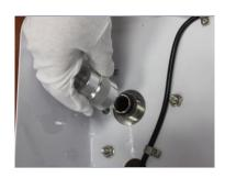
Step 10: Install the earth wire to the base.
