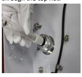
**Step 3:** Remove the top and bottom nuts from the **UV** chamber
