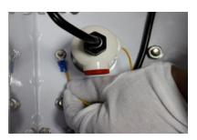
**Step 11:** Use the plastic wrench if you want to change the filter. Apply Trevoli Super-O-lube food grade lubricant to the filter O-rings.
