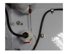
Step 4: Insert the Quartz sleeve into the Reactor Chamber.
